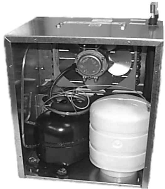
Evaporator installed (Back view of unit)
